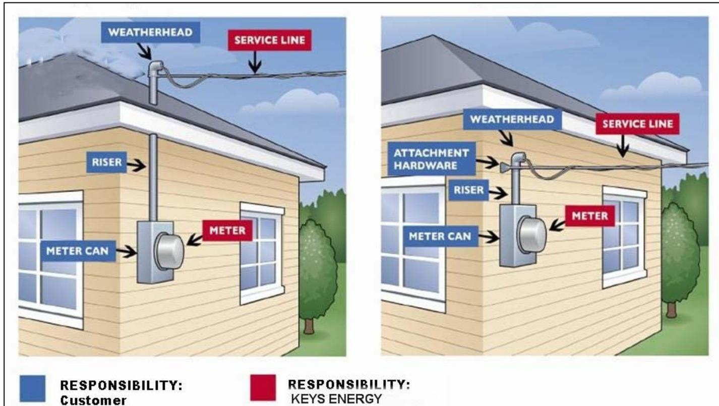
The diagram on the right illustrates a meter center that no longer meets current electrical codes. If/when this type of meter center is replaced, KEYS customers will have to update their facilities to reflect the diagram on the left.
